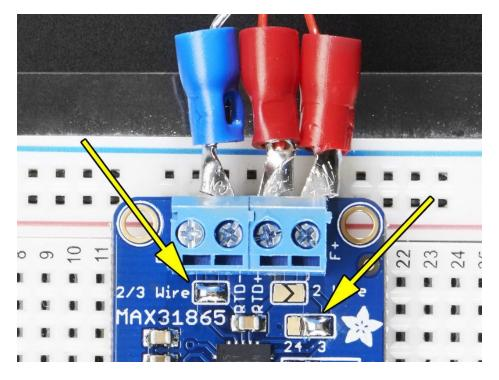
You will have to cut the thin trace in between the 2-way jumper on the right side of the board, and then solder closed the blob on the right side.
