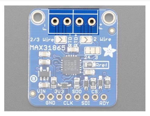
If you have an RTD sensor, you need to connect it somehow! the terminal block area is where you can clamp down to the sensor wires.
