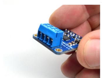
Next we will solder in the two 3.5mm terminal blocks used to connect power & the motor to the breakout board.
