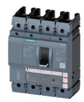
circuit breaker 3VA5 UL frame 250 breaking capacity class H 65kA @ 480V 4-pole, line protection TM210, FTFM, In=175A overload protection Ir=175A fixed short-circuit protection Ii=10 x In N conductor protection 100% without connection
