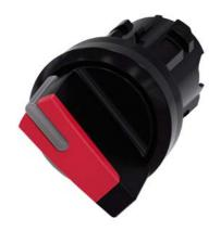
Selector switch, illuminable, 22 mm, round, plastic, red, selector switch, short, 2 switch positions O-I, latching, actuating angle 90°, 10:30h/13:30h, with laser labeling, lower case
