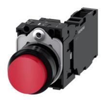
Pushbutton, 22 mm, round, plastic, red, pushbutton, raised, momentary contact type, with holder 1 NO+1 NC, screw terminal, with laser labeling, upper case and lower case, always upper case at beginning of line
