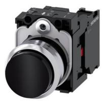
Pushbutton, 22 mm, round, metal, shiny, black, pushbutton, raised, momentary contact type, with holder, 1 NC, screw terminal, with laser labeling, inscription or symbol Customer-specific selection with SIRIUS ACT configurator (CIN)
