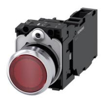
Illuminated pushbutton, 22 mm, round, metal, shiny, red, pushbutton, flat, momentary contact type, with holder, 1 NO+1 NC, LED module with integrated LED 24 V AC/DC, screw terminal, with laser labeling, inscription or symbol Customer-specific selection with SIRIUS ACT configurator (CIN)
