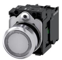
Illuminated pushbutton, 22 mm, round, metal, shiny, clear, pushbutton, flat, momentary contact type, with holder, 1NO, LED module with integrated LED 24 V AC/DC, screw terminal, with laser labeling, symbol number according to, ISO 7000 or IEC 60417
