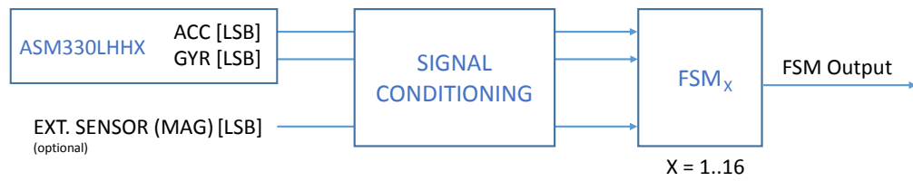
Figure 2. State machine in the ASM330LHHX
