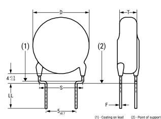
(1) - Coating on lead shall not extend below this line.
