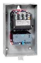
Non-reversing motor starter, Size 1, Three phase full voltage, Solid-state overload relay, OLR amp range 3-12A, 24VAC 50-60Hz coil, Non-combination type, Enclosure type 1, Indoor general purpose use, Extrawide enclosure
