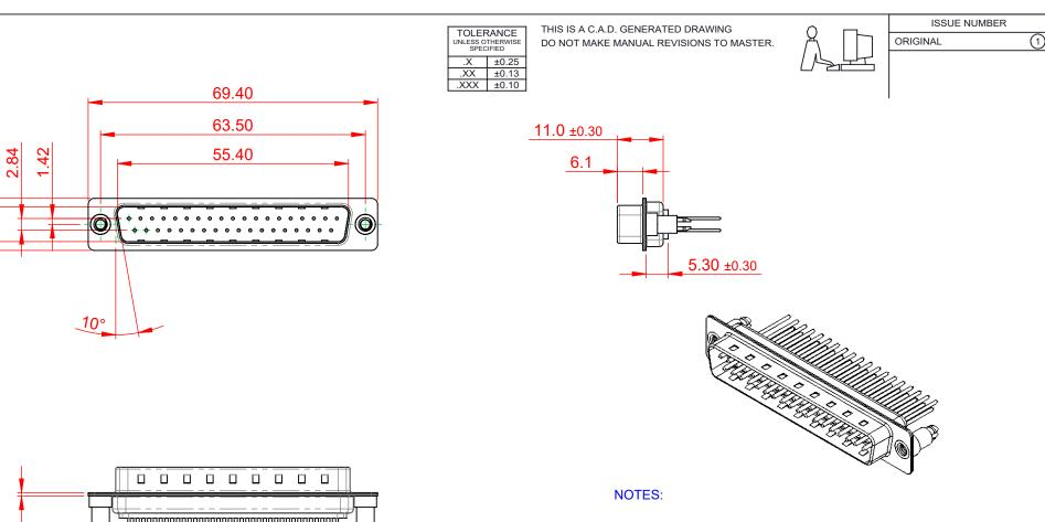
MATERIAL: HOUSING: WHITE THERMOPLASTIC POLYESTER, UL94V-0 SHELL: STEEL, NICKEL PLATED CONTACT: COPPER ALLOY, 30µ GOLD PLATED
