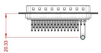
POWER/CO-AX CONTACT RATING:40A (CURRENT)(IF PRESENT)SIGNAL CONTACT CURRENT RATING:5A PER CONTACTSIGNAL CONTACT RESISTANCE:10mΩ MAX.INSULATOR RESISTANCE:5000MΩ min.DIELECTRIC5000MΩ min.
