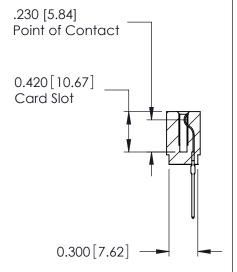
725 Series Ultra-Mate Card Edge Connector - Press Fit Part Number: 725-027-545-101
