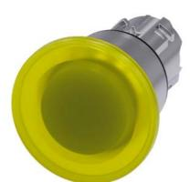
Illuminated mushroom pushbutton, 22 mm, round, metal, shiny, yellow, 40 mm, latching, pull-to-unlatch mechanism, with laser labeling, upper case and lower case, always upper case at beginning of line
