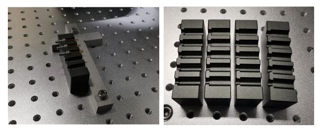
3. 2D Laser marking sample photos2D marking size is 2mm x 2mm.
