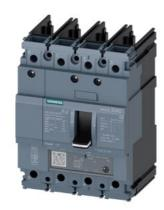
circuit breaker 3VA5 UL frame 125 breaking capacity class H 65kA @ 480V 4-pole, line protection TM230, FTAM, In=125A overload protection Ir=125A fixed short-circuit protection Ii=5...10 x In N conductor unprotected without connection
