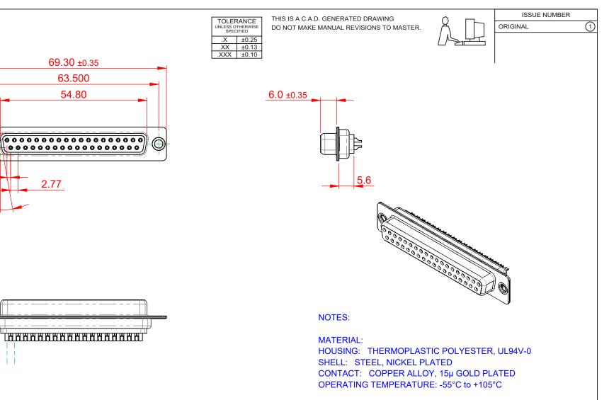
CURRENT RATING: 3A PER CONTACT CONTACT RESISTANCE:  $25m\Omega$  MAX. INSULATOR RESISTANCE:  $5000M\Omega$  min. DIELECTRIC WITHSTANDING VOLTAGE: 1000V AC rms
