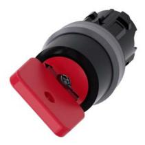
Key-operated switch O.M.R, 22 mm, round, plastic with metal front ring, lock number 73037, red, with 2 keys, 2 switch positions O<I, momentary contact type, Actuating angle 45°, 10:30h/12h, key removal O, with laser labeling, inscription or symbol Customer-specific selection with SIRIUS ACT configurator (CIN)
