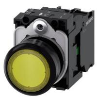
Illuminated pushbutton, 22 mm, round, plastic, yellow, pushbutton, flat, momentary contact type, with holder, 1NO, LED module with integrated LED 230 V AC, screw terminal, with laser labeling, lower case
