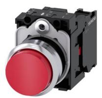
Pushbutton, 22 mm, round, metal, shiny, red, pushbutton, raised, momentary contact type, with holder, 1 NC, screw terminal, with laser labeling, upper case and lower case, always upper case at beginning of line
