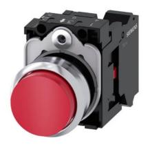
Pushbutton, 22 mm, round, metal, shiny, red, pushbutton, raised, momentary contact type, with holder, 1 NC, spring-type terminal, with laser labeling, symbol number according to, ISO 7000 or IEC 60417
