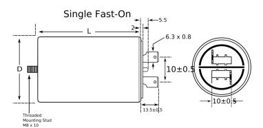
General Information Series C27 Dielectric Film/Foil Polypropylene Style Plastic Case and Cover, Ultra Sonically Welded Description Ultra Sonically Welded Seal, Safety Class PO, Features UL 94 V0 Disk **RoHS** Yes Lead Fast On (1+1) UL, VDE, UL (Construction Only), UL\_94 VO Qualifications Disk AEC-Q200 No Component 142 g Weight
