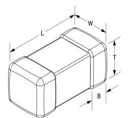
SeriesL-RMSStyleSMD ChipDescriptionSurface Mount InductorRoHSYesCoreCeramicWinding TypeMultilayer
