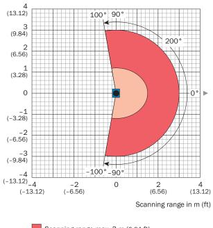
Scanning range max. 3 m (9.84 ft) Scanning range 1.2 m to 1.5 m (3.94 ft to 4.92 ft) for objects with 10 % remission, dependent on the angle
