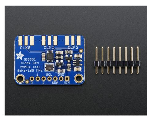
The Si5351 clock generator is an I2C controller clock generator. It uses the onboard precision clock to drive multiple PLL's and clock dividers using I2C instructions. By setting up the PLL and dividers you can create precise and arbitrary
