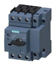
Circuit breaker size S00 for motor protection, CLASS 10 with overload relay function A-release 10...16 A N-release 208 A screw terminal Standard switching capacity
