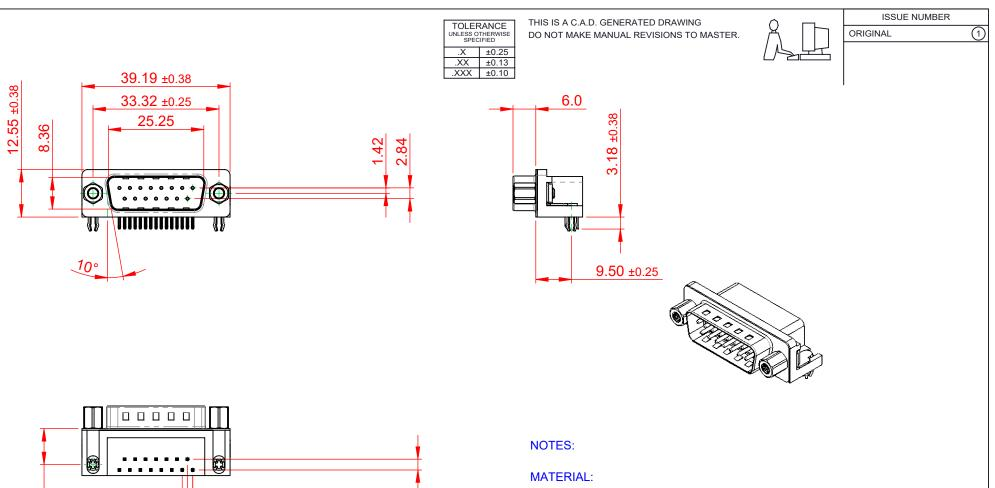
HOUSING: SHELL: CONTACT: THERMOPLASTIC POLYESTER, UL94V-0 STEEL, NICKEL PLATED COPPER ALLOY, 15µ GOLD PLATING
