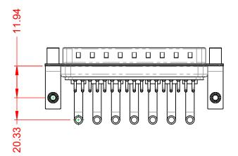
30A (CURRENT) POWER/CO-AX CONTACT RATING: (IF PRESENT) SIGNAL CONTACT CURRENT RATING: 5A PER CONTACT SIGNAL CONTACT RESISTANCE:  $10m\Omega$  MAX. **INSULATOR RESISTANCE:** 5000MΩ min. DIELECTRIC
