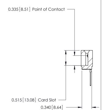
ACAD REFERENCE NO. 746-ENG MASTER 746 Series Ultra-Mate Card Edge Connector - Press Fit DRAWN: J.LEE DATE: AUG 20/09 Part Number: 746-022-545-101 CHECKED: DATE: **EDAC INC** SCALE: SHEET 1 OF 1 THESE DRAWINGS AND SPECIFICATIONS ARE THE PROPERTY OF EDAC INC.,AND TORONTO, ONTARIO SHALL NOT BE REPRODUCED, OR COPIED DRAWING NUMBER CANADA OR USED AS THE BASIS FOR THE 746-ENG MASTER MANUFACTURE OR SALE OF APPARATUS YOUR CONNECTION TO QUALITY & SERVICE WITHOUT WRITTEN PERMISSION.
