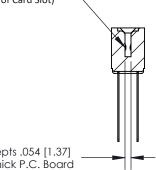
Card Slot Accepts .054 [1.37] to .070 [1.78] Thick P.C. Board
