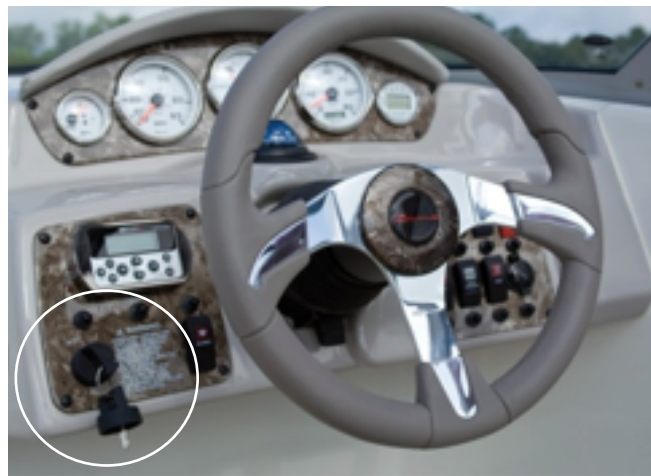
95060 Ignition Switch in an exposed position on the dash of a Stingray boat
