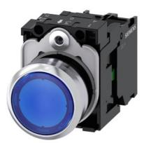
Illuminated pushbutton, 22 mm, round, metal, shiny, blue, pushbutton, flat, momentary contact type, with holder, 1NO, LED module with integrated LED 24 V AC/DC, screw terminal, with laser labeling, lower case
