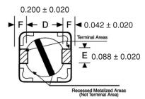
HRSPD73 Height Dimension 'C' 0.166 Inches Max (4.20 mm Max) **HRSPD73** Terminal Dimensions  $0.190 \pm 0.005$  'D' (in) by  $0.100 \pm 0.010$  'F' (in)
