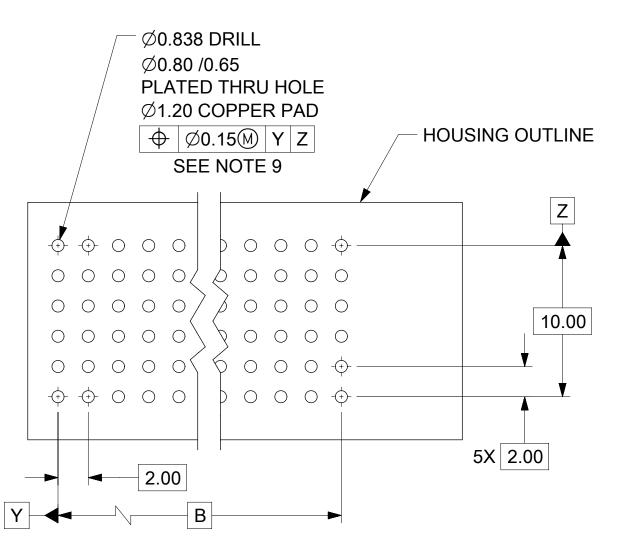
PCB LAYOUT : COMPONENT SIDE RECOMMENDED PCB THICKNESS: 2.50 MIN.
