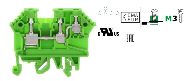
Feed-through terminal, Screw connection, Mounting type:Mounting rail TS 35/7.5 and TS 32, Rated cross-section: 4 mm², Width: 6 mm, Colour: Green
