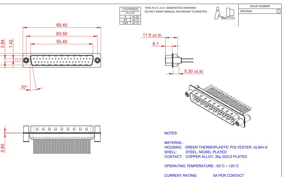
CONTACT RESISTANCE:  $25m\Omega$  MAX. INSULATOR RESISTANCE: 5000MΩ min. DIELECTRIC WITHSTANDING VOLTAGE: 1000V AC rms
