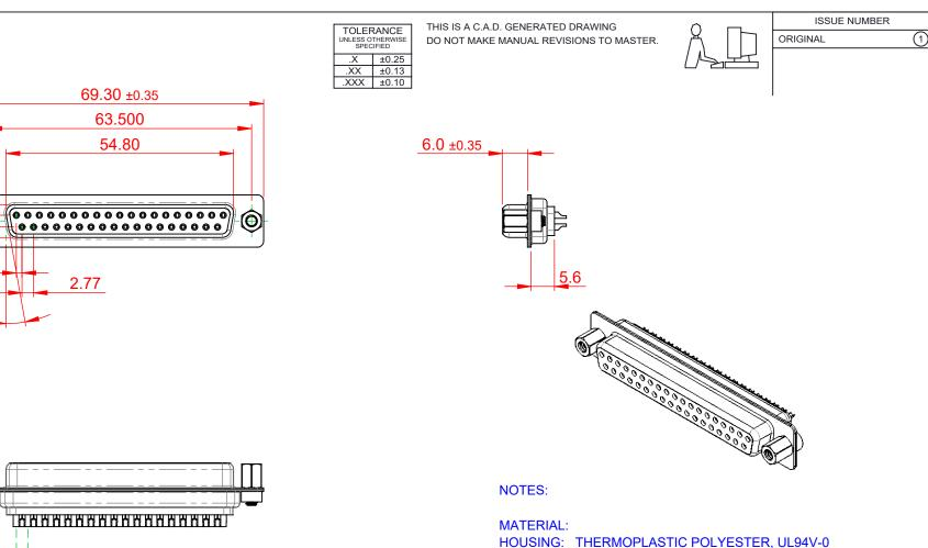
HOUSING: THERMOPLASTIC POLYESTER, UL94V-0 SHELL: STEEL, TIN PLATED CONTACT: COPPER ALLOY, 15µ GOLD PLATED OPERATING TEMPERATURE: -55°C to +105°C
