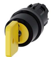
Key-operated switch O.M.R, 22 mm, round, plastic, lock number 73033, yellow, with 2 keys, 3 switch positions I-O-II, latching, actuating angle 2x45°, 10:30h/12h/13:30h, Key removal I+O+II, with laser labeling, inscription or symbol Customer-specific selection with SIRIUS ACT configurator (CIN)
