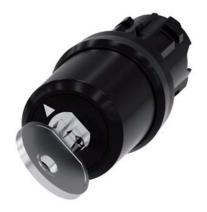
key-operated switch Siemens, 22 mm, round, plastic, lock number SSG10, with 2 keys, 2 switch positions O-I, latching, actuating angle 90°, 10:30h/13:30h, key removal I, with laser labeling, upper case and lower case, always upper case at beginning of line
