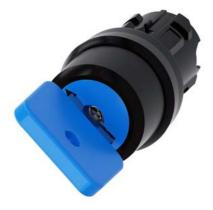
Key-operated switch O.M.R, 22 mm, round, plastic, lock number 73038, blue, with 2 keys, 2 switch positions O<I, momentary contact type, Actuating angle 45°, 10:30h/12h, key removal O, with laser labeling, upper case and lower case, always upper case at the beginning of the word
