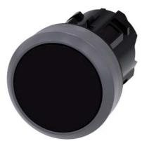
Pushbutton, 22 mm, round, plastic with metal front ring, black, pushbutton, flat, latching, Push-to-release mechanism, with laser labeling, symbol number according to, ISO 7000 or IEC 60417
