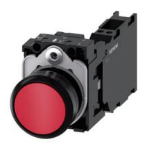
Pushbutton, 22 mm, round, plastic, red, pushbutton, flat, momentary contact type, with holder 1 NO+1 NC, spring-type terminal, Z=20-unit packaging
