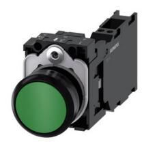
Pushbutton, 22 mm, round, plastic, green, pushbutton, flat, momentary contact type, with holder 1 NO+1 NC, spring-type terminal, with laser labeling, upper case and lower case, always upper case at the beginning of the word
