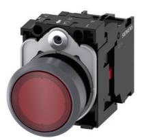
Illuminated pushbutton, 22 mm, round, plastic with metal front ring, red, pushbutton, flat, momentary contact type, with holder, 1NC, LED module with integrated LED 230 V AC, screw terminal, with laser labeling, upper case
