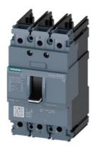
circuit breaker 3VA5 UL frame 125 breaking capacity class S 25kA @ 480V 3-pole, line protection TM210, FTFM, In=110A overload protection Ir=110A fixed short-circuit protection Ii=10 x In UL 489 SB (naval),  $50^\circ$  C without connection
