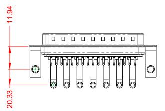
POWER/CO-AX CONTACT RATING:30A (CURRENT)(IF PRESENT)SIGNAL CONTACT CURRENT RATING:5A PER CONTACTSIGNAL CONTACT RESISTANCE: $10m\Omega$  MAX.INSULATOR RESISTANCE: $5000M\Omega$  min.DIELECTRICDIELECTRIC
