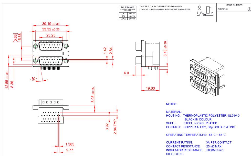
WITHSTANDING VOLTAGE: 1000V AC rms
