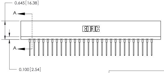
737 Series Ultra-Mate Card Edge Connector - Press Fit ACAD REFERENCE @TION - ACAD REFERENCE
