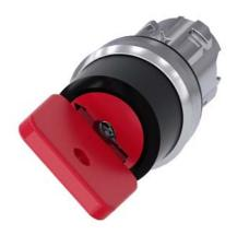
Key-operated switch O.M.R, 22 mm, round, metal, shiny, lock number 73037, red, with 2 keys, 2 switch positions O-I, latching, actuating angle  $90^{\circ}$ , 10:30h/13:30h, key removal O+I, with laser labeling, lower case
