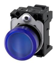
Indicator lights, 22 mm, round, plastic, blue, lens, smooth, with holder, LED module, with integrated LED 24 V AC/DC, spring-type terminal, with laser labeling, symbol number according to, ISO 7000 or IEC 60417
